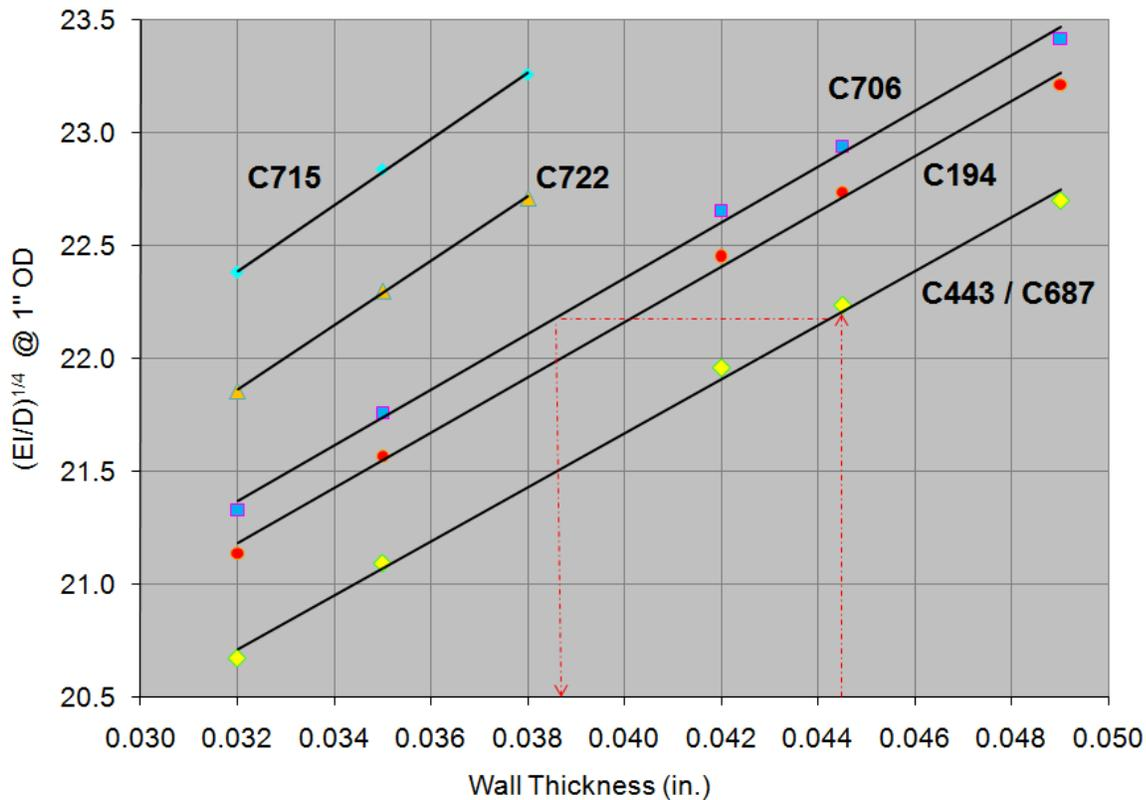
Figure 2 –  $(EI/D)^{1/4}$  for 1.000" OD Tubes plotted vs. Wall Thickness.
