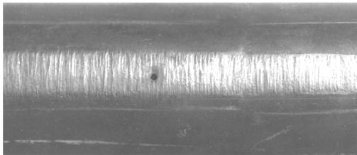
Figure 1 – Through-wall perforation resulting from mid-span collision.
