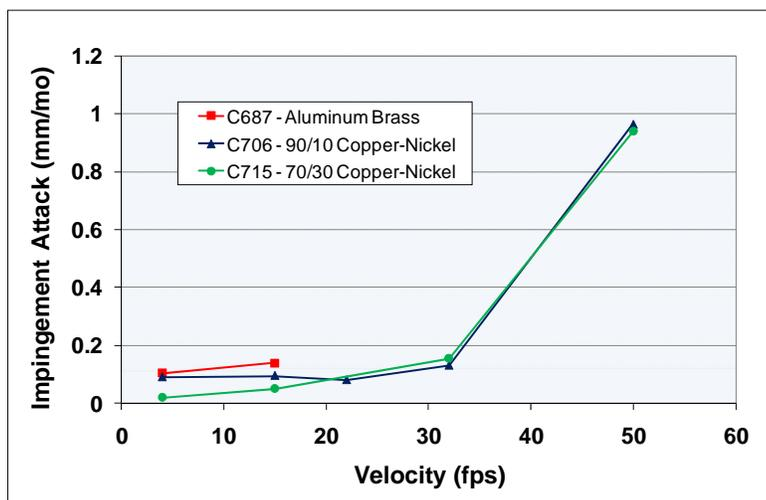
**Figure 3 – Jet Impingement Attack at Varying Water Velocities**
