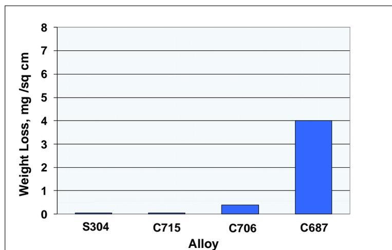
**Figure 1 - Weight loss of various alloys after exposure to 1000 ppm NH<sub>3</sub> contaminated condensate at 38C (100F) for 10 days <sup>(5)</sup>.**
