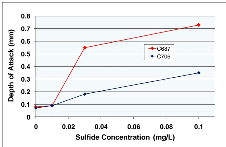
**Figure 2 – The Effect of Sulfides on the Pitting Corrosion of 90/10 Copper-Nickel and Aluminum Brass at 7 m/sec at 5-20 °C <sup>(9)</sup>.**
