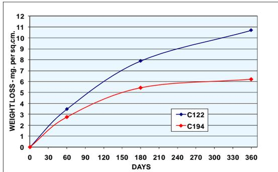
**Figure 1 – Corrosion of Alloys C194 and C122 in New Haven Potable Water at 7fps.**
